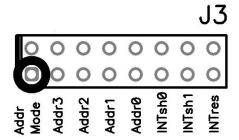
The address range for the board itself is directly selected by the Addr3, Addr2, Addr1 and Addr0 jumper locations. The following table describes the base addresses of the controllers 0 and 1 (CAN 0 and CAN 1) for every possible combination of Addr Mode and AddrX jumper locations.
